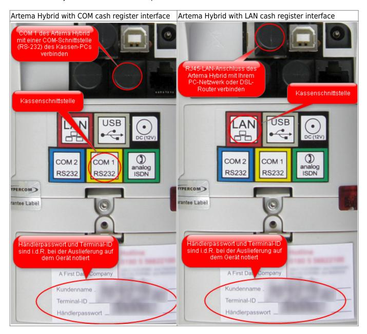
The connections of an Artema Hybrid are shown here. The arrangement of the interfaces may differ for your terminal.
