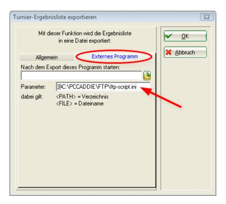
Parameters for calling up the \*.ini file which then triggers the upload.
