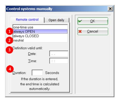
1. Here you have the option of opening or keeping a door closed once or permanently, for example. The one-off opening can be password-protected if required.
