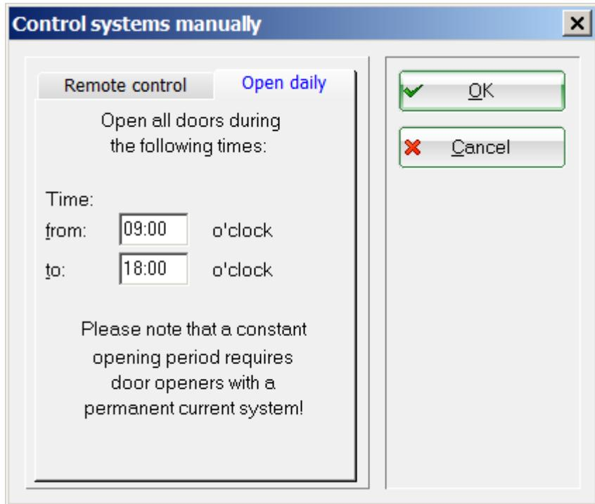
! Please note that the electric strike must be designed for continuous current for permanent opening.
